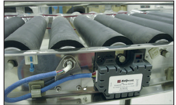
Figure 2 Motorized rollers in a BLDC conveyor
